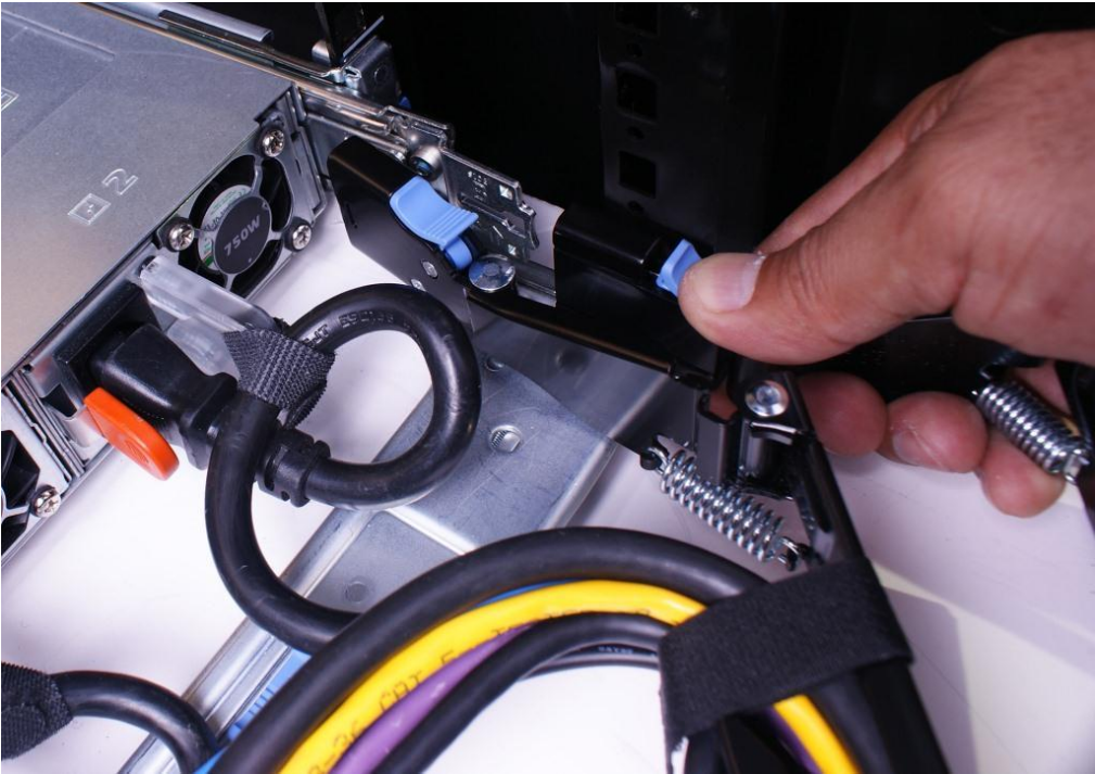
Figure 7. Disconnecting the CMA attachment housings
