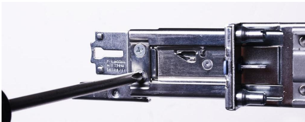
Figure 10. Removing the outer CMA brackets for shallow racks
